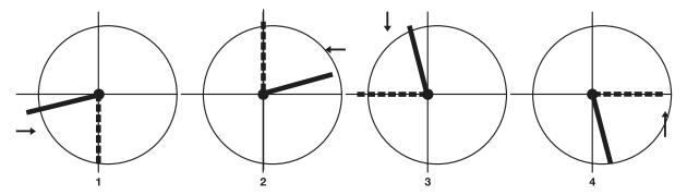
Typical vane orientations — arrows indicate direction of flow Solid vane shows "off" positions
